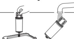
**4 Insert the cartridge into the funnel and press in into position (until it stops)**
